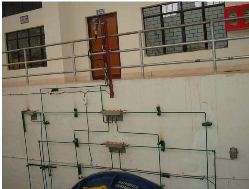
Figure 4: Differential pressure transducer installed for relative discharge measurement for the index test
