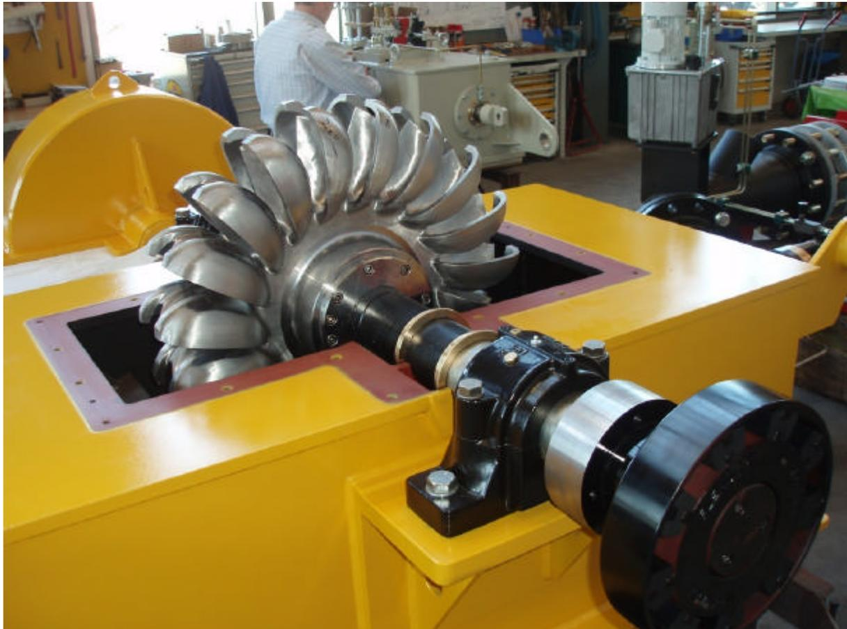
Figure 4.3 Turbine runner with housing at Wasserkraft Volk's premises
